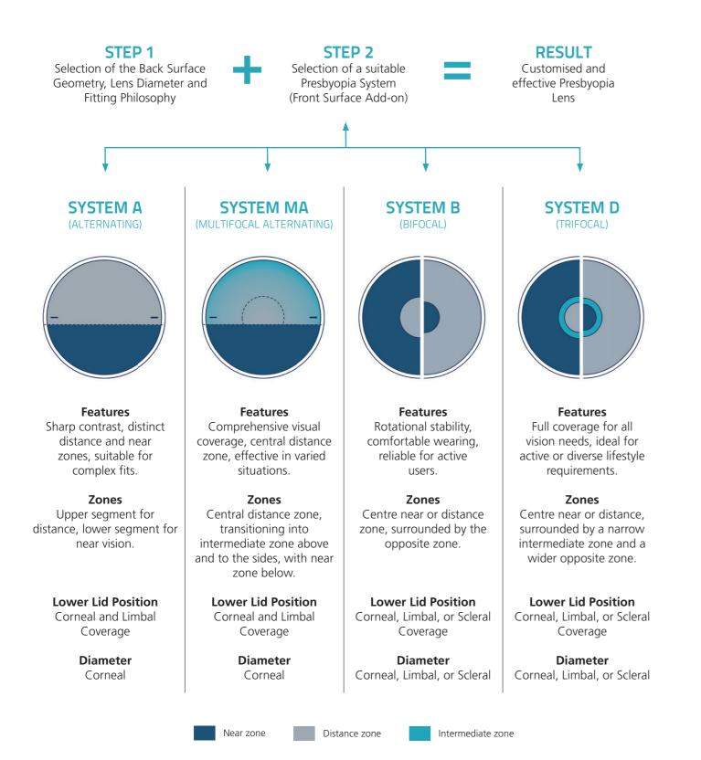
All presbyopia systems are modular and can be integrated with any lens design, including toric lenses for astigmatic corrections with cylinders in all axis positions.
